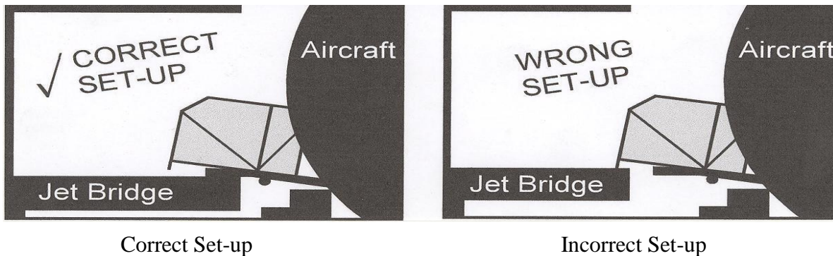
Figure 3 – Side View of Set-up, Air Stair with folding handrails.
