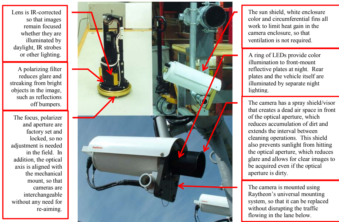
Figure 3.4.6-3 Camera Assembly. The Raytheon Camera Assembly is designed for toll collection image capture. All other gantry-mounted equipment uses a similar mounting and cabling design with captive screws and environmental connectors.
