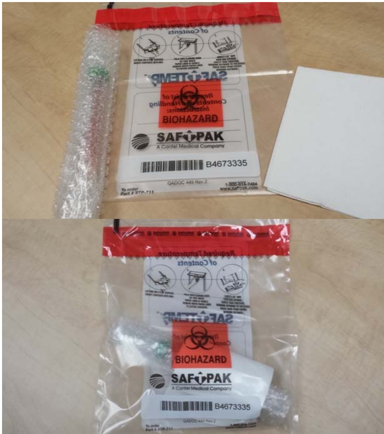
Figs. 3a-b: 3a (top) shows the cushioned primary receptacle alongside the secondary receptacle, along with absorbent material. 2b (bottom) shows the secondary receptacle sealed. In this case, the secondary receptacle, when properly sealed, is rated to withstand a maximum pressure differential of 9k kPa, making it suitable for shipping Biological Substances, Category B.
