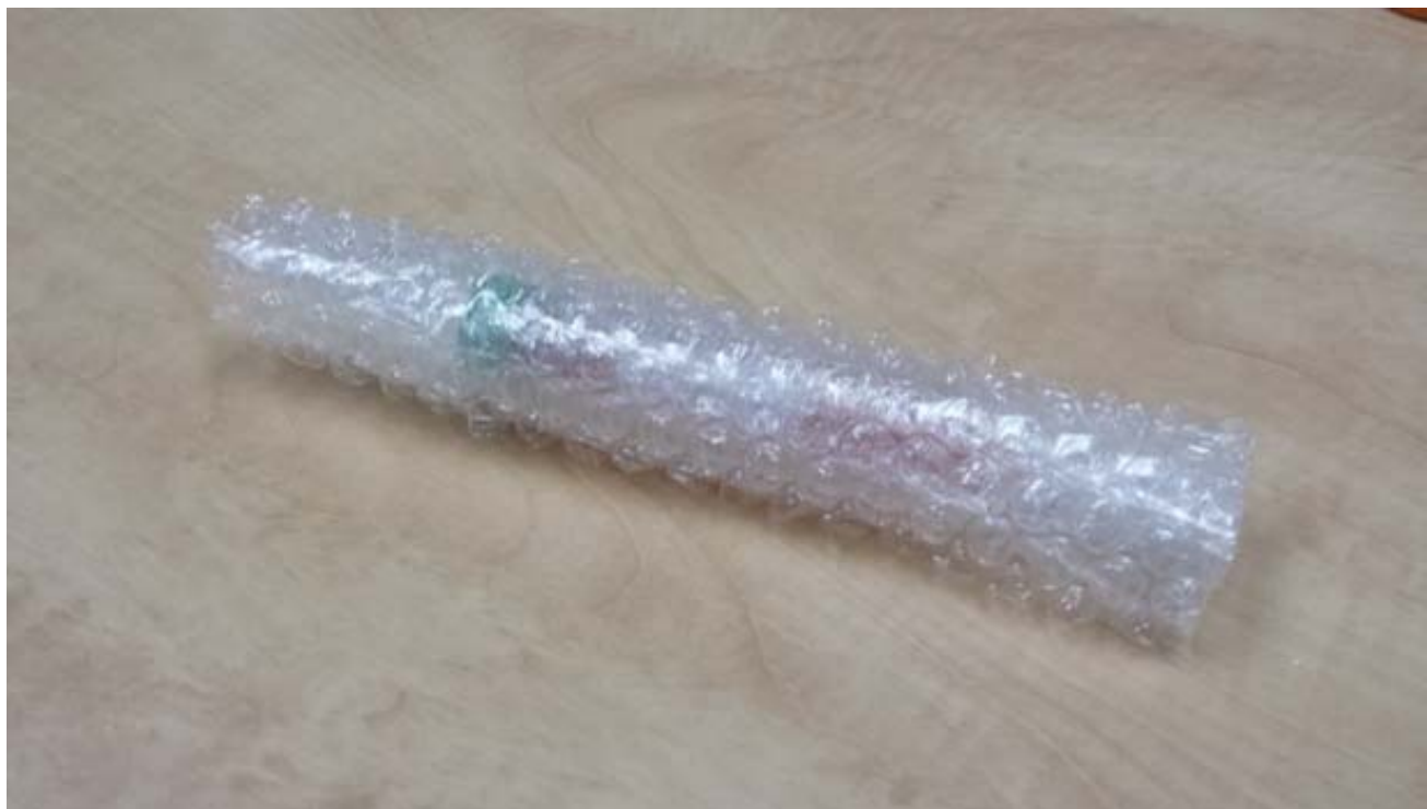
Figs. 2a-b: 2a (top) shows a 15 mL screw-top tube, an acceptable primary receptacle. 1b (bottom) shows the primary receptacle individually wrapped in bubble wrap to cushion it during transport.
